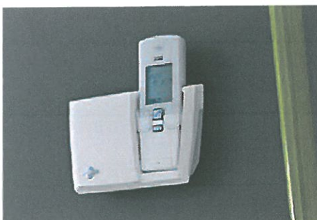
Wall mounted handset with lithium battery power pack base (mains not required)
